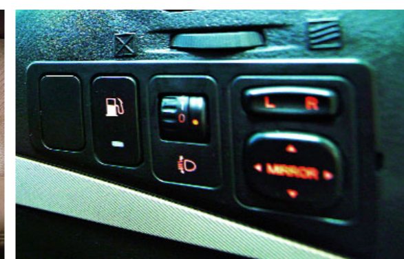
This cluster of switches on the driver's side houses the fuel lid, headlight and mirror adjustment switches.
